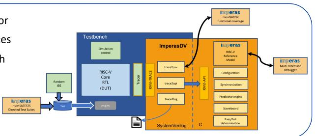
ImperasDV, with asynchronous continuous compare methodology, is needed to support features such as interrupts, privilege modes, Debug mode, multi-hart, multi-issue and OoO pipeline, ...
